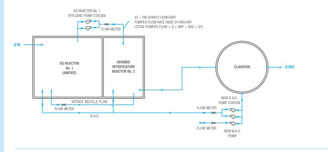
Bardenpho Diagram for EquaReact<sup>®</sup> 5 stage BNR and enhanced Bio P Removal
